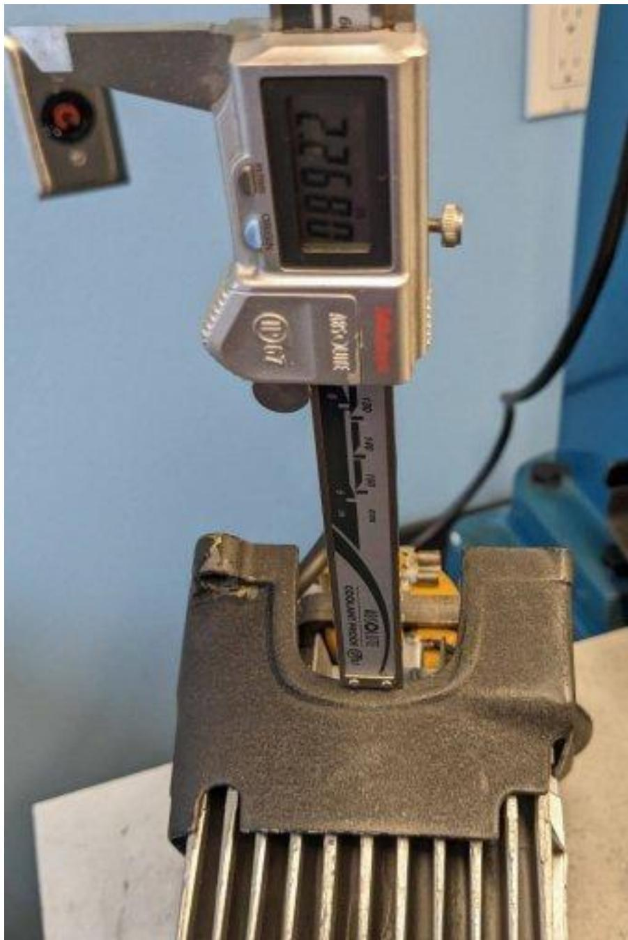
Push the piston to bottom dead center -- insert the caliper and zero -- roll slowly up to and thru top dead center -- the reading should be 1.442" (=- .003") -- (this value is slightly longer than the stated stroke value (1.375" max) since the measurement is being taken on an angle)
