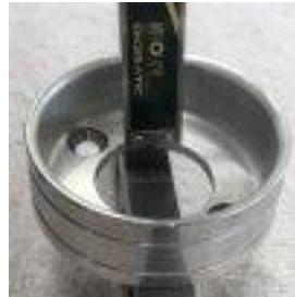
**136.4.** remove head -- install dial indicator and using the LAD inspection tool -- check exhaust height (1.155") and inlet height (0.775")
