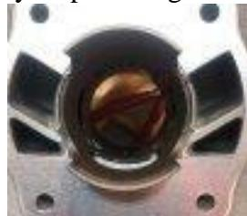
**136.8.** check piston pin -- 0.420" maximum inside diameter
