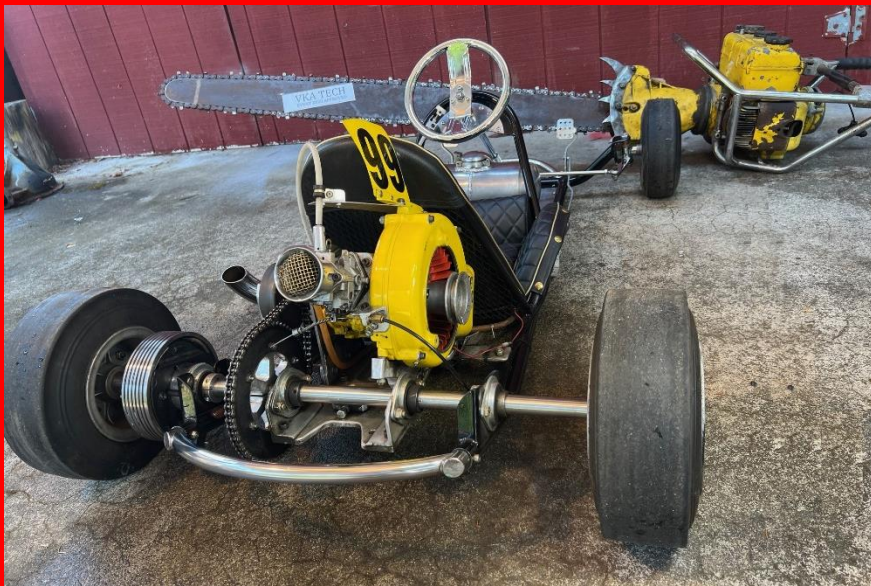
1958 reproduction (my first Kart); U-Weld-It Flex Products kit ($9.75); with 1954 McCulloch 99 rotary valve 9.8ci. 2-man saw. Nils Gustafson, Wilderville, Oregon.
