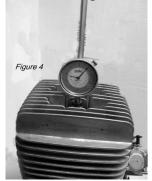
**135.4** With the head removed, measure the cylinder bore diameter using calipers -- Maximum bore is 2.100"
