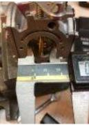
136.2.2 remove carb gasket and check inlet track for 2.600" minimum length
