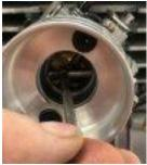
**136.2.1** remove carb and check throttle bore 1.010" no-go
