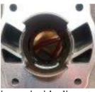
136.8 check piston pin -- 0.420" maximum inside diameter
