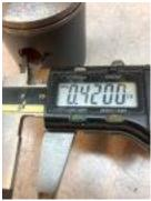
**136.9** use no-go gauge to check exhaust --max overall width 1.551" max --- rib 0.140" min
