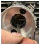
**136.2.1** remove carb and check throttle bore 1.010" no-go
